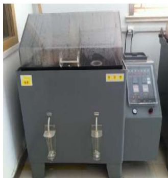
盐雾腐蚀箱 Salt spray Chamber
